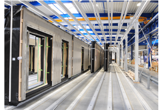
The wall modules produced by Nokera await their deployment at the construction site.
